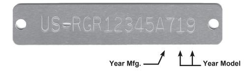
The hull I.D. Plate is located on the outboard side of the starboard transom, above the water line, and contains the following information:
