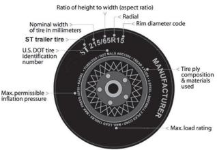
**Maximum Permissible Inflation Pressure:** Indicates the tire manufacturer's maximum permissible pressure and/or the pressure at which the maximum load can be carried by the tire. Refer to the Certification Label on the port forward half of the trailer for the correct tire pressure for your trailer.
