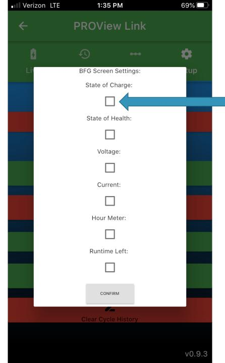
On screen setting click at a minimum state of charge and voltage to display
