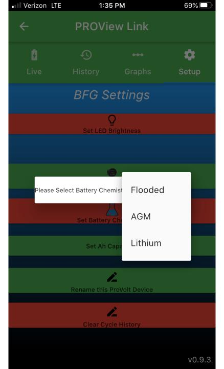
Select Battery Chemistry, input either AGM or Lithium depending on BOM. BFG is programmed to default to Lithium. Trolling motor will always be Lithium option
