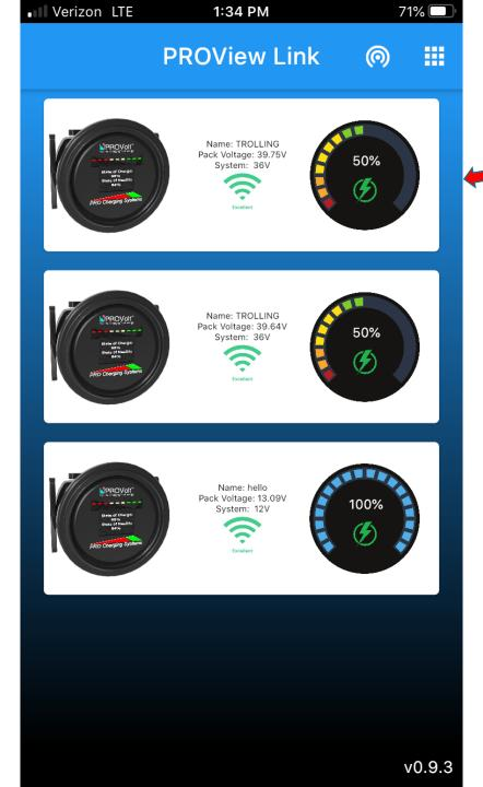
Click on top gauge, 12 V system will open crank portion of BFG, 36 V system will open trolling portion of BFG. Crank and Trolling are on separate PCBs and are controlled independently through the app
