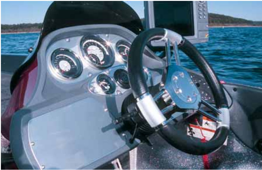
The helm is as attractive as it is functional. Note the Teleflex Pro Trim switch on the steering column, which made it easy to adjust engine trim and jackplate height.
